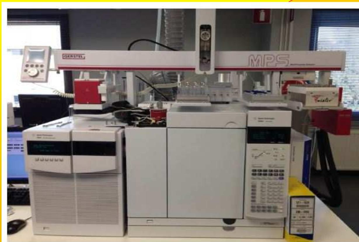
Determination of volatile aldehyde compounds in samples using PFBOA impregnated PDMS tubes, DHS sampling and GCMS analysis in SIM-mode :
