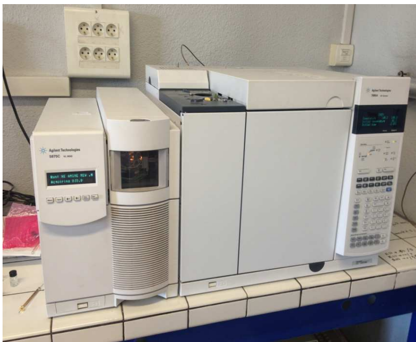
Fig 6. Agilent Technologies GC 7890A with MS 5975C VL MSD
